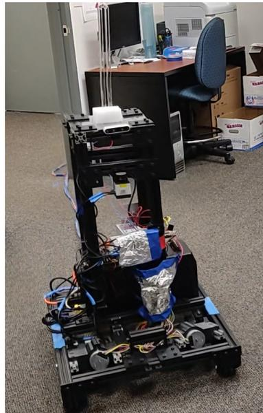
Fig. 2. The robot developed for autonomous UVC irradiation driving into a room to be disinfected.
