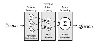
Figure 1: Basic schema-based reactive architecture
