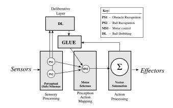
Figure 3: Integration of schema-based reactive layer and simple deliberative layer using the GLUE component
