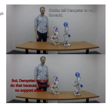
**Figure 1:** Dempster (blue) is given the goal to walk forward via Shafer (red). Dempster begins to carry out the goal, but fails when the edge of the table is detected. This goal failure is then reported from Shafer's perspective.
