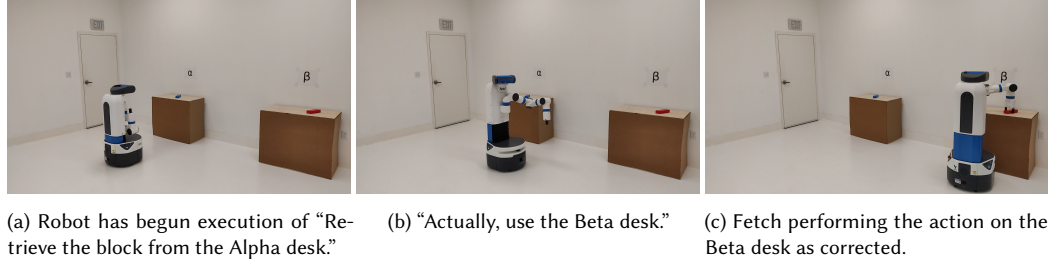
Fig. 2. Action script correction during execution. The left desk is labeled “Alpha” and the right desk is labeled “Beta”.
