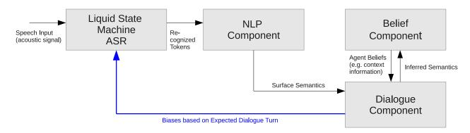
Figure 1: Information flow through the natural language system. The blue arrow indicates the top-down dialogue context bias on the ASR component introduced in this paper.
