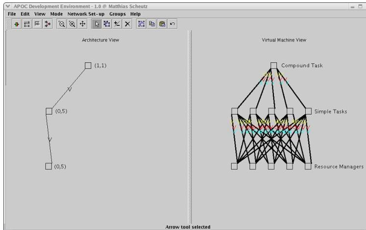
Figure 1: ADE Interface: The left side shows the types of components which can be present in the architecture and their possible interconnections. The right side shows the components (boxes) and communication paths (lines) in the running virtual machine
