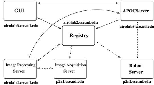
Figure 2: ADE Set-up for ball retrieval in the robot experiment
