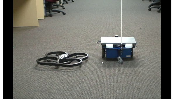
Figure 2. The quadricopter (left) and Videre (right) robotic platforms utilized for the study 4 .
