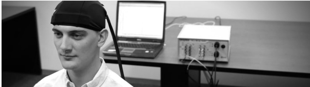
Figure 1. fNIRS sensors secured to forehead with a tight cap tethered to ISS OxiplexTS tissue oximeter next to the laptop computer.
