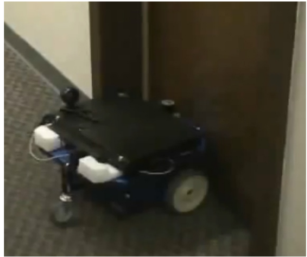
Figure 2: A Videre ERA equipped with a USB web-cam, a Hokuyo Urg laser range-finder, a microphone, and a quad-core Linux PC for onboard processing exercising its newly-acquired capability of opening closed doors to look for red boxes.
