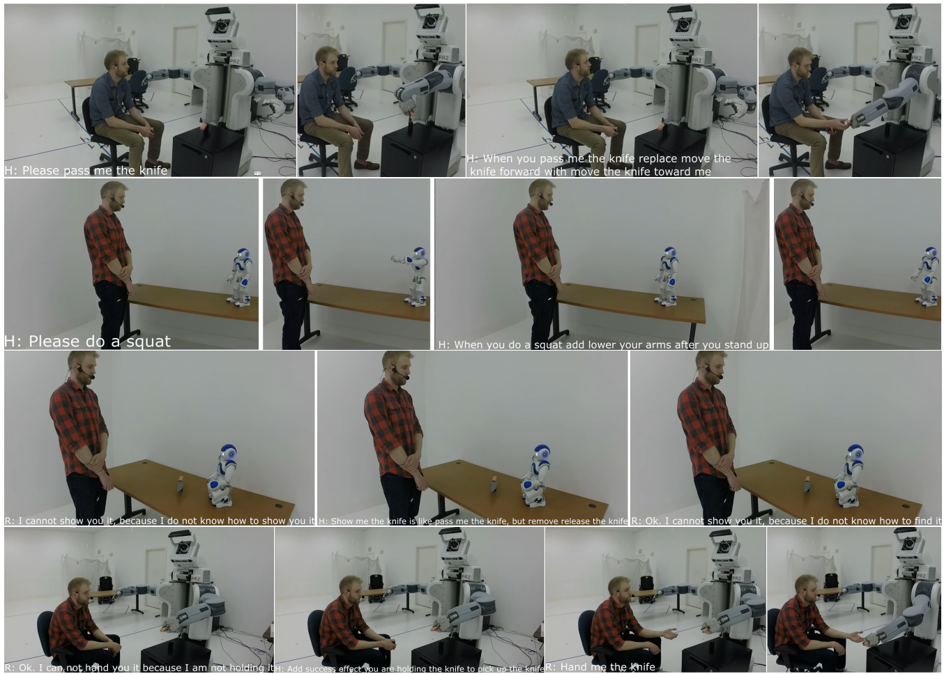
Figure 1: First row: When passing the knife the robot moves the knife forward, Brad tells it to move the knife toward him instead. Second row: The robot performs the squat action and Brad notices it didn't lower its arms. He repairs the action by telling the robot to lower its arms after standing up. Third row: The robot doesn't know show the knife. Brad tells the robot that show is similar to passing a knife, however don't release it. Fourth row: Asking the robot to hand over the object, which the robot knows how to perform, but it requires that it holding the knife. The robot doesn't understand that it is holding the knife when it picks it up. Brad instructs the robot that it is indeed holding the knife.
