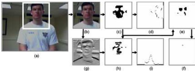
Fig. 2. A diagram of the Analogical CNN Algorithm.
