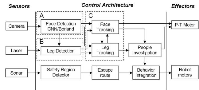
Fig. 1. The basic architecture for people tracking. The dashed areas indicate separate, concurrently operating subsystems for face detection (A), leg detection (B), and face and leg tracking, respectively (C).
