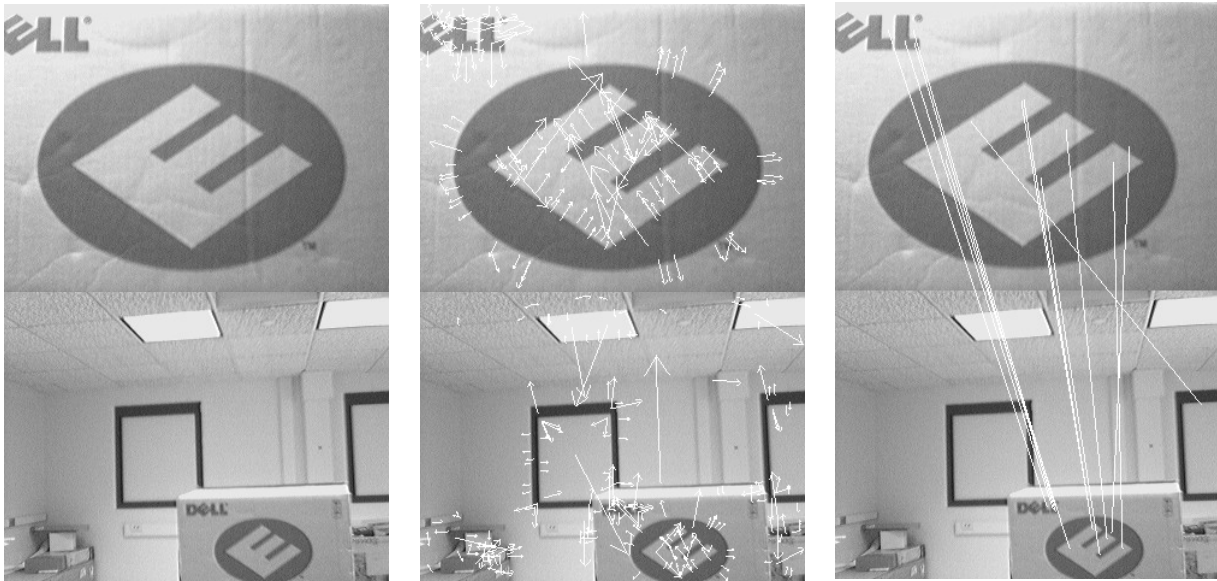
Figure 3: Left: Unprocessed training (top) and scene (bottom) images. Center: SIFT points located during individual processing. Right: SIFT point matches detected when comparing the two images.
