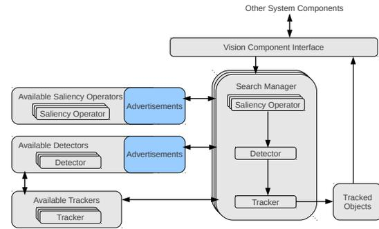
Figure 1: The processing architecture of the vision system.
