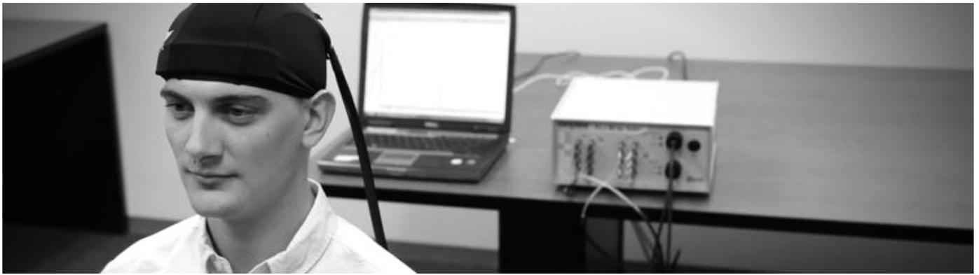
Fig. 2. NIRS equipment and physical setup. Participant is fitted with two NIRS sensors, secured by a tight-fitting cap, and tethered to the NIRS oximeter (behind, right) and a laptop for data recording.
