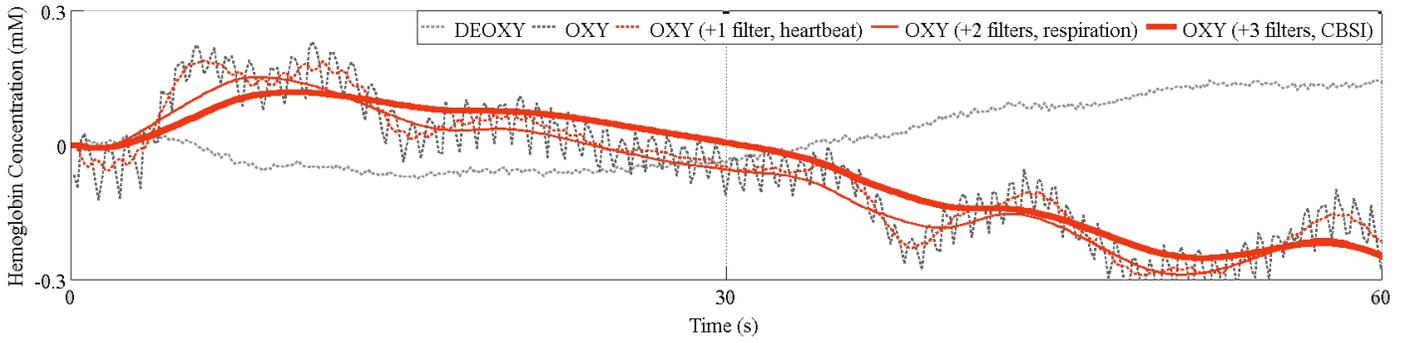
Fig. 3. Signal processing. Heartbeat artifacts are first filtered with a lowpass filter between 0.6Hz and 2Hz. From the resulting signal, respiration is removed. Finally, CBSI is applied to the denoised signal (shown in red, bold). The resulting signal shows the inverse correlation between oxy and deoxy measures.
