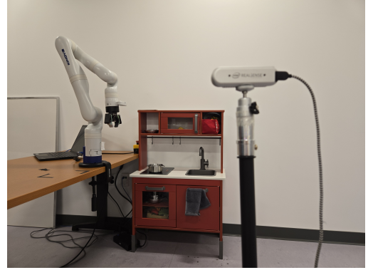
Fig. 2: Deployment environment. The Kinova 7-DoF arm (visible on the left), can reach all elements of the kitchen play set (center). An Intel RealSense camera (right) captures the full scene.
