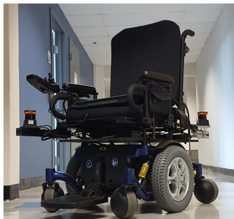
Figure 1: The Vulcan Intelligent Wheelchair: one of the robot platforms used in the presented work.
